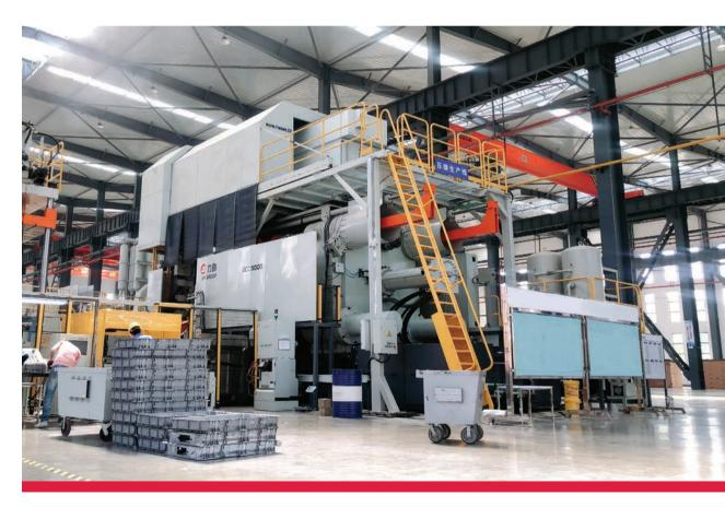
Impress-Plus Large Tonnage Die-Casting Machine (5000T):
