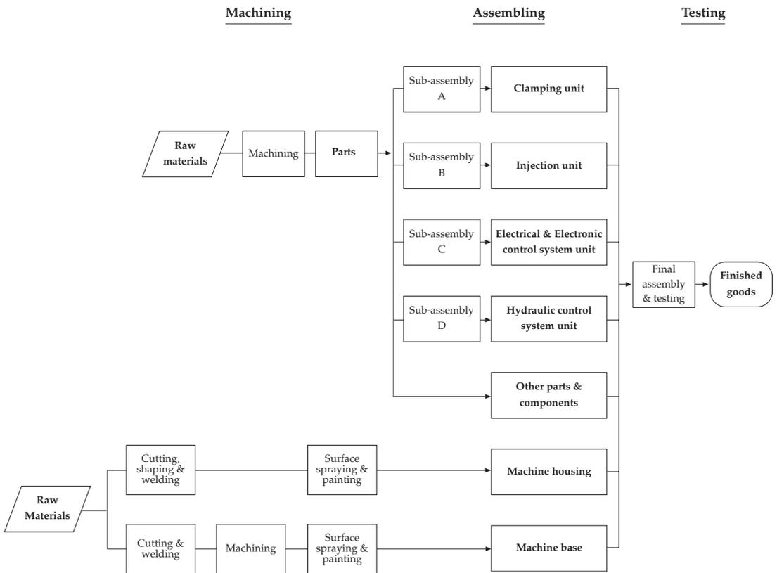
The production of the Group's products mainly involve three major steps, namely machining, assembling and testing.
