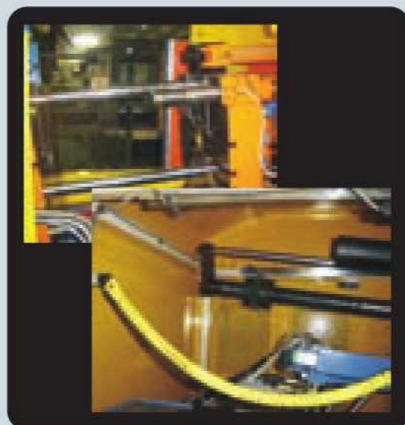
Hydraulic Tie Bar Extraction
