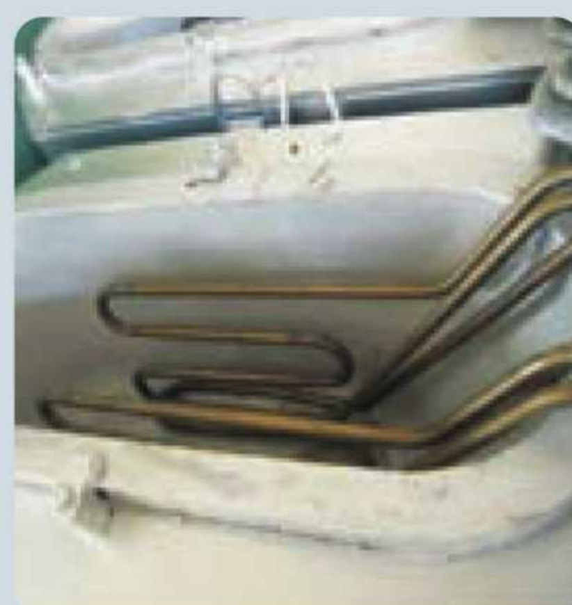
Immerse type electrical heating device for furnace
